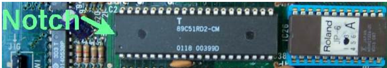
Figure 13 – Europa chip shown installed – Notched end to the LEFT!
